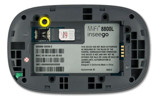
Insert or remove a nano SIM card by pressing down the tab and sliding the nano SIM card with the gold contacts facing the Jetpack.
