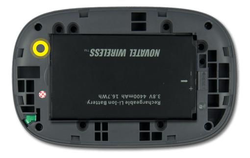
Align the gold contacts on the side of the battery to the gold contacts inside the battery compartment and set the battery in place.
