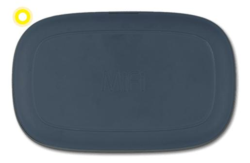
Put the back cover on by pressing down on along the edges until it snaps into place.
