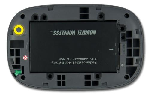
Remove the battery by placing a fingernail in the release notch on the side of the battery compartment and lifting it toward you.
