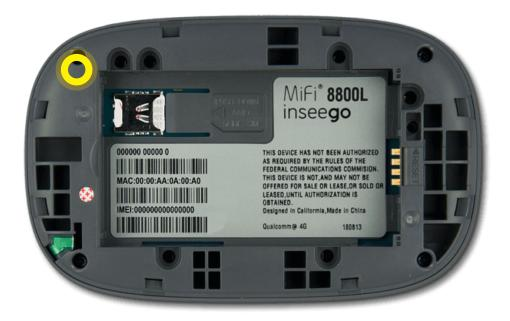
Remove the nano SIM card cover by pressing down the release tab and sliding the nano SIM card out of the Jetpack.
